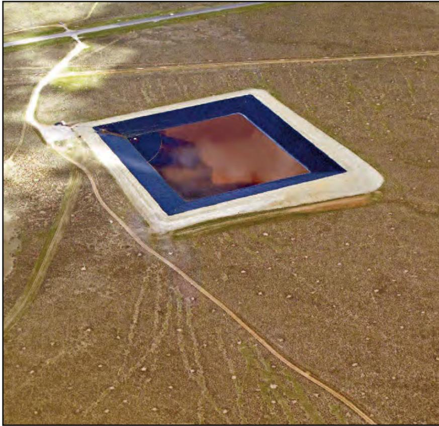
An aerial image of a "produced" water evaporation pond in Pavillion, WY, where the mixture of water, sand and chemicals used in fracking is stored after it's brought back to the surface.
