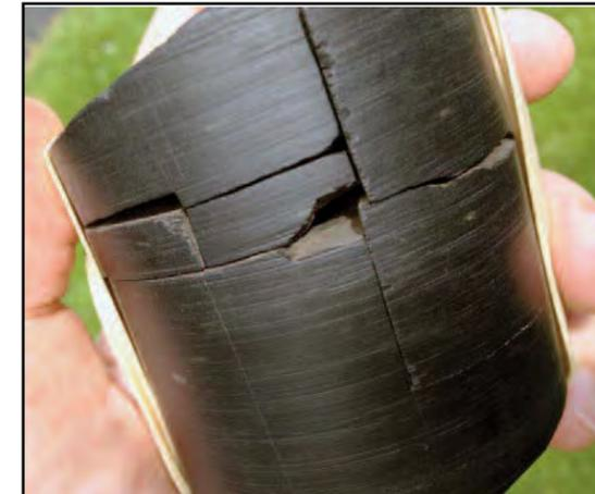
A section of Marcellus shale that's been fracked. Deep under the earth, fracking opens fissures in the shale that allow oil and gas to seep into the hole left behind from drilling. The gas is then pumped up and out of the well.
